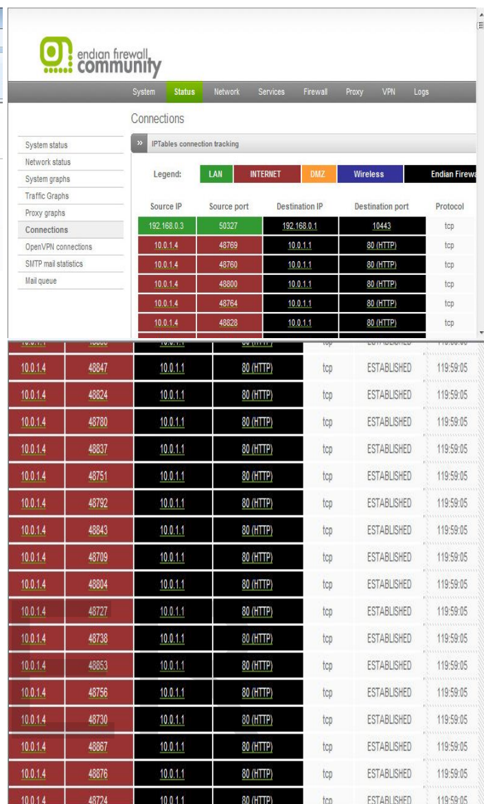
Figure 6.6 Detection of Dos Attack by Firewall
